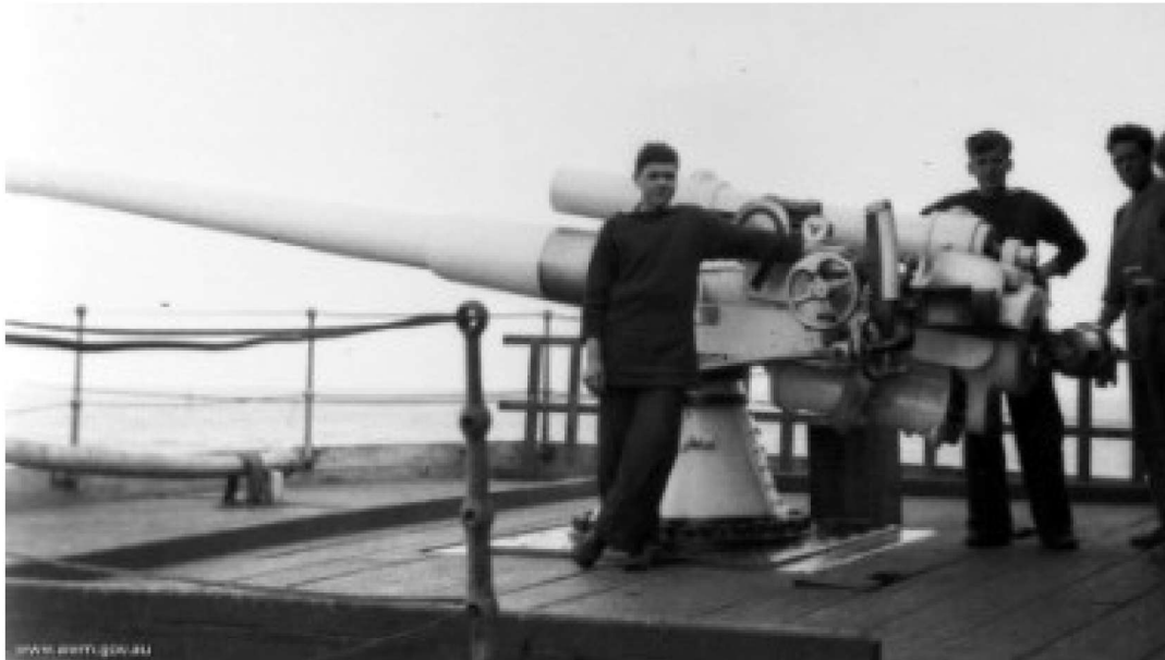
Figure 2 QF 4.7" Mk V* Naval gun and crew on the S.S. ORCA, 1919
